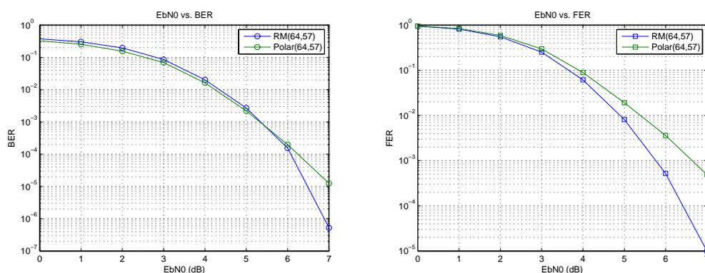
Figure 1: Error rates for (64,57) polar and RM codes on a BPSK channel.
