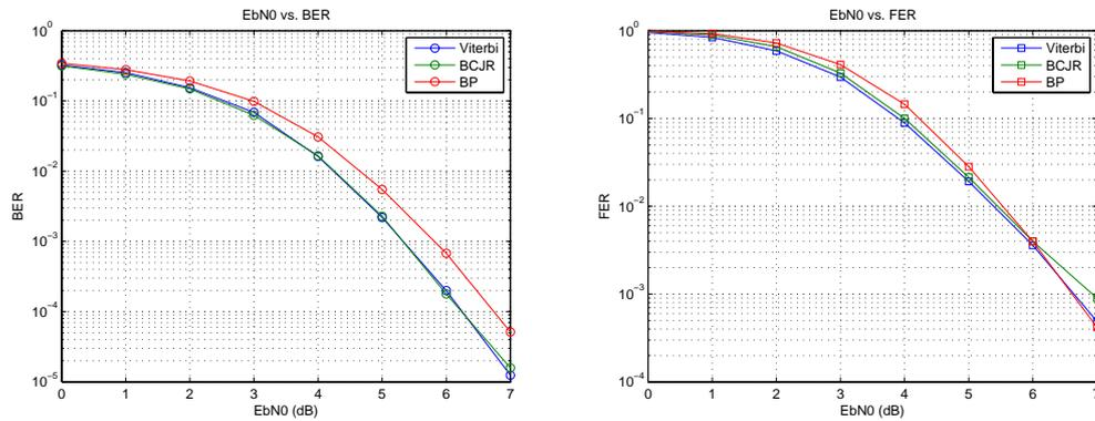
Figure 2: Error rates for the (64,57) polar code under various decoding algorithms.
