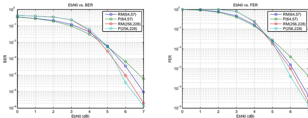
Figure 3: Error rates for polar and RM codes of sizes (64,57) and (256,228) under BP decoding on a BSPK channel.
