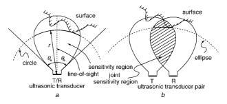
Fig. 1 Ultrasonic transmission and reception
