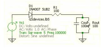
Perform a transient analysis by hand calculation on the above circuit and obtain the voltage-time plots for 3 periods, for the voltage of the output. Show your work clearly along with the associated equations. Assume the capacitor voltage to be zero before t=0,  $V_{s1}$  is a square wave with 5V amplitude, 2.5V DC offset and also the  $f_{osc}$ =100 kHz.
