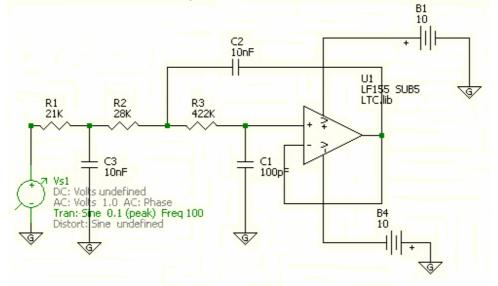
The capacitor  $C_3$  has an initial voltage of 1V. You may need to modify the circuit to put the initial condition.
