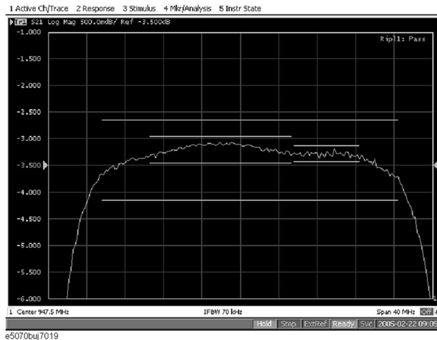
**NOTE** The individual frequency bands for the ripple test can overlap each other; in this case, the ripple limit test is performed for each frequency band.
