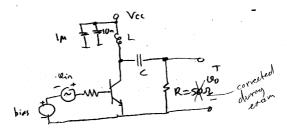
A power amplifier as shown above is operated at 100 MHz. It is driven to function in class-B mode. The transistor  $T_1$  can handle 2A and 20V as maximum current and voltage respectively without being damaged.
