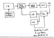
The block diagram of a PLL circuit is given above. The reference oscillator frequency is 10 MHz. The operating frequency range of the PLL is 500-600 MHz. The channel spacing is 100kHz. Maximum possible phase detector frequency is used in the system.
