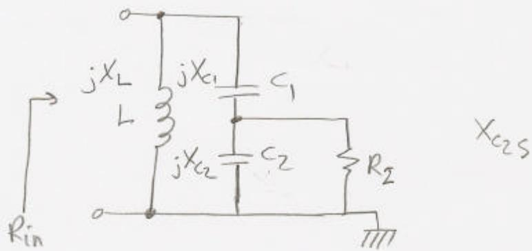
In this circuit we would like to find the impedance seen in parallel with the inductor, namely  $R_{in}$ . The problem is similar to  $\pi$ -match, with differences:
