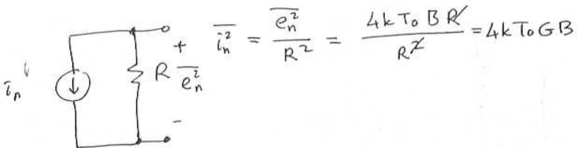
For  $10 \text{ kHz}$  BW  $\left( \frac{10000 \text{ Hz}}{1 \text{ Hz}} \right)^{1/2} = 100$
