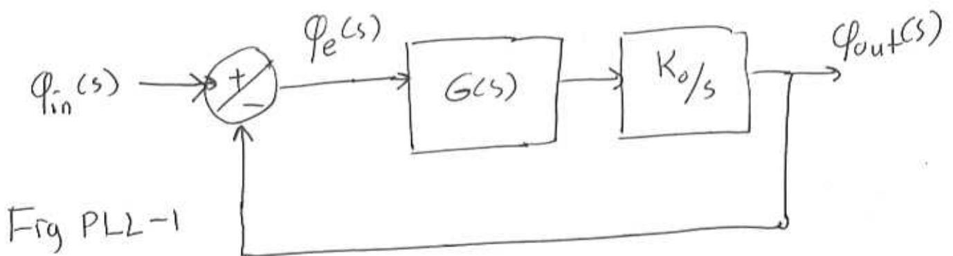
$G(s)$  is the gain function of the loop filter
