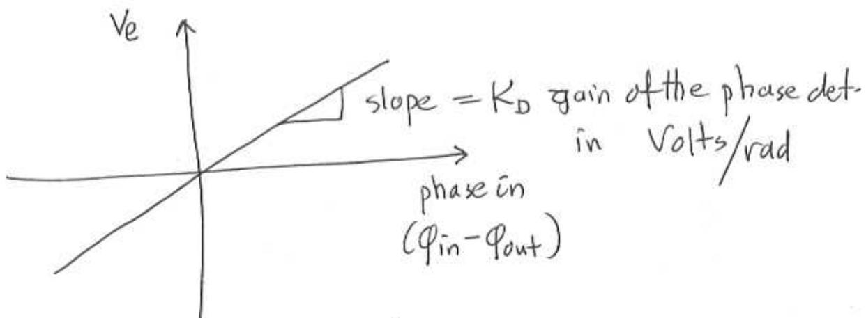
The characteristics of an ideal Phase Detector assumed at the analysis. The relationship between the phases and frequencies are defined as follows:
