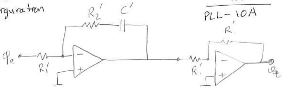
$$\frac{\omega_t}{R_2' + \frac{1}{sC'}} = \frac{\phi_e}{R_1'} \Rightarrow \frac{\omega_t}{\phi_e} = \frac{R_2' + \frac{1}{sC'}}{R_1'}$$
