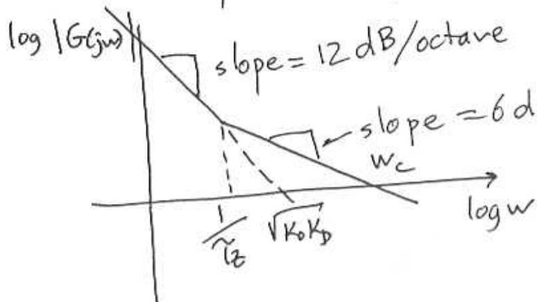
$\omega_c$  is the cross over frequency of the open-loop gain
