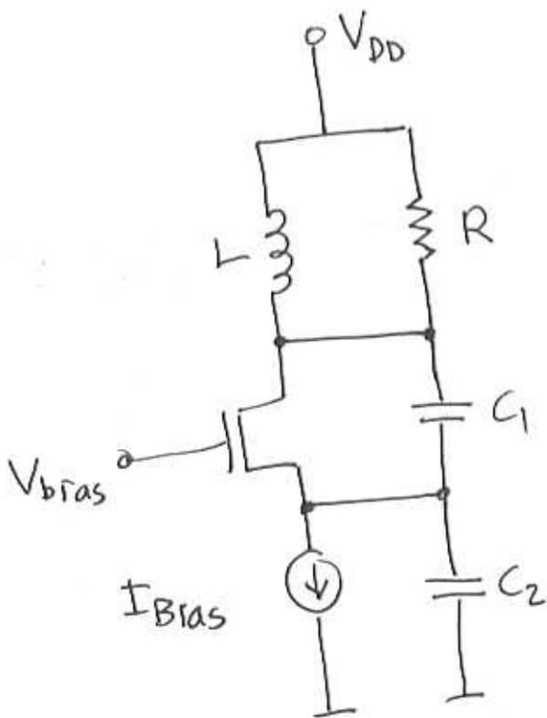
The series combination of  $C_1$  &  $C_2$  creates a tank circuit (parallel RLC) with  $L$  loaded by  $R$ .
