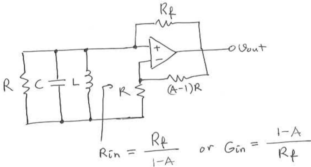
If the conductance loading the tank circuit is negative then an oscillation starts. Therefore:
