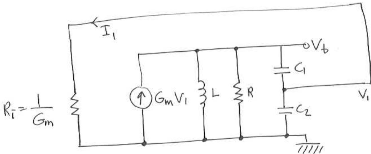
As the amplitude of the oscillation increases, the input impedance (the source impedance) increases, decreasing the large-signal admittance which is equal to the large-signal transconductance. Assuming that, there was enough gain margin at the small-signal model, i.e. the final oscillation amplitude is large enough to switch the transistor on and off at each cycle and the conduction angle is small enough, the bias current and the fundamental current driving the tank circuit can be related as:
