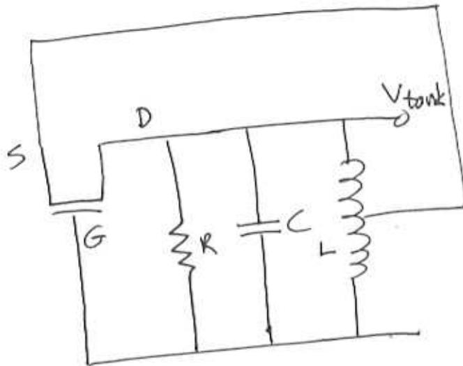
Hartley is a colpitts like oscillator where an inductive divider instead of a capacitive voltage divider is used.
