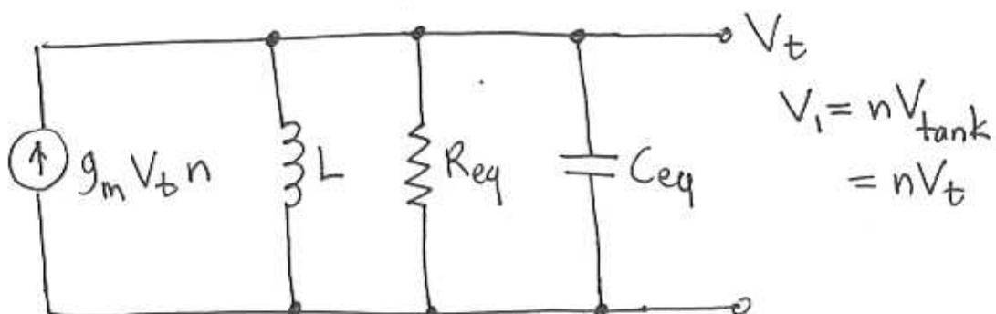
$$R_{eq} = R // \frac{1}{n^2 g_m} \quad n = \frac{C_1}{C_1 + C_2} \quad C_{eq} = \frac{C_1 C_2}{C_1 + C_2} \quad \omega = \frac{1}{\sqrt{L C_{eq}}}$$
