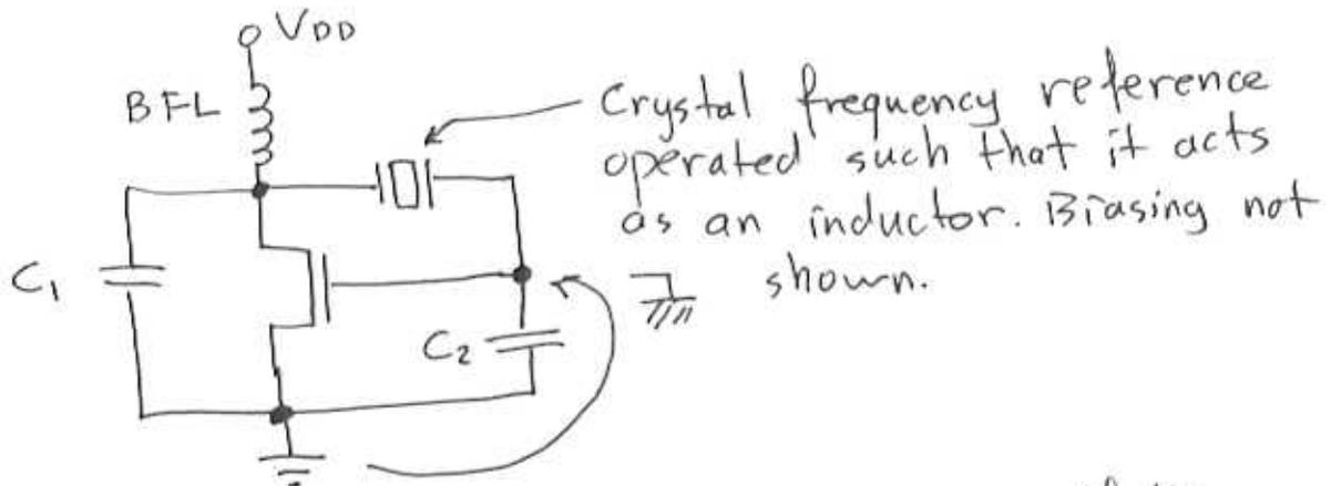
The circuit is grounded at the source. If the ground is moved to the gate, which does not affect the operation of the circuit, then circuit becomes a colpitts oscillator as shown below.
