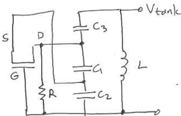
Clapp is a modified colpitts oscillator where the tank has an additional capacitive divider. The Q of the tank must be calculated taking the additional divider into account.
