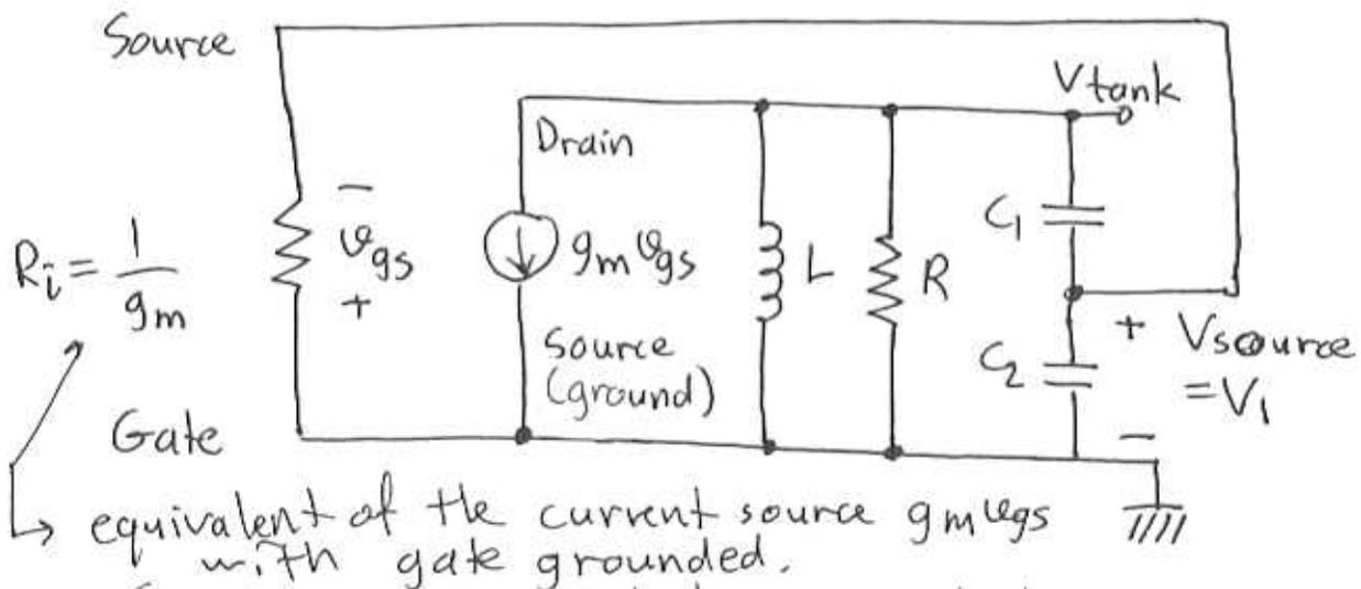
Source is connected to ground because the other side of a current can be connected to any other place without disturbing the tank circuit.
