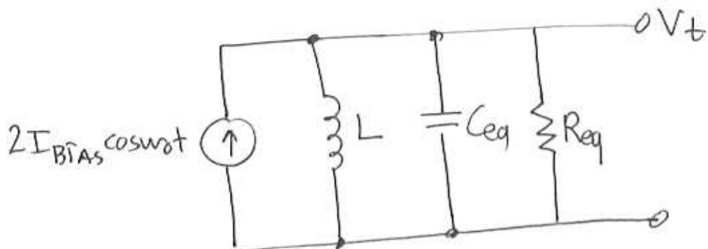
$$G_m = \frac{I_1}{V_1} = \frac{2I_{BIAS}}{V_1} \quad V_1 = n V_{\text{tank}}$$
