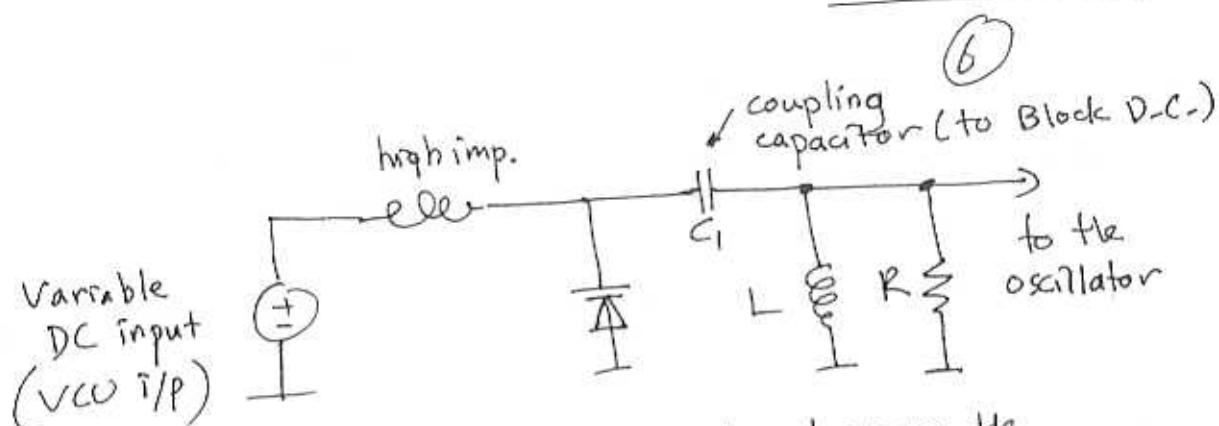
Sometimes  $C_1$  is used to decrease the capacitor range to a suitable value and also to absorb some of the voltage on the varactor to limit the AC voltage on the varactor. A more practical circuit is
