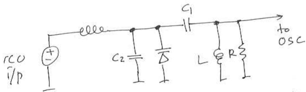
Suitable values of  $C_1$  &  $C_2$  maps the varactor range to the required capacitor range whilst manipulating the AC swing on the varactor to minimize the effects of the nonlinearity of the varactor.
