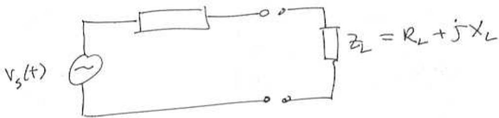
Find  $Z_L$  such that maximum power is transferred to the load for a given  $Z_s$ .
