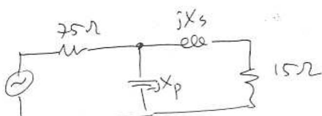
$$Q_{\text{loaded}} = \frac{Q_{\text{match}}}{2} = \frac{2}{1} = 1 = \frac{75 // 75}{37.5} = \frac{R_P}{X_P}$$
