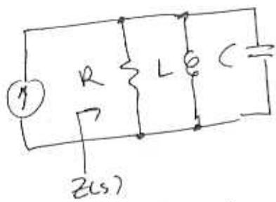
The natural response is determined by the zeroes of the admittance or the poles of the impedance  $Z(s)$
