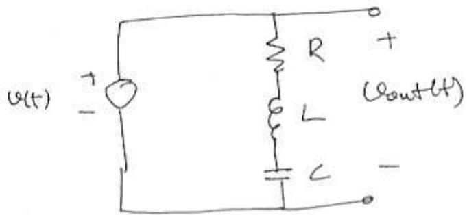
Almost the same kind of equations are used except  $Q$  is given in a different form as the dual of the parallel RLC circuit
