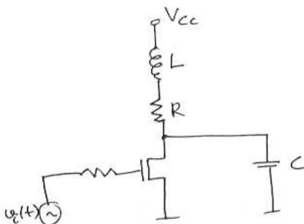
The o/p time constant is  $RC$  which creates a 3dB cut-off frequency  $\omega_c = \frac{1}{2\pi RC} = \frac{1}{2\pi \tau_c}$ , for  $L = 0$ . The question is:
