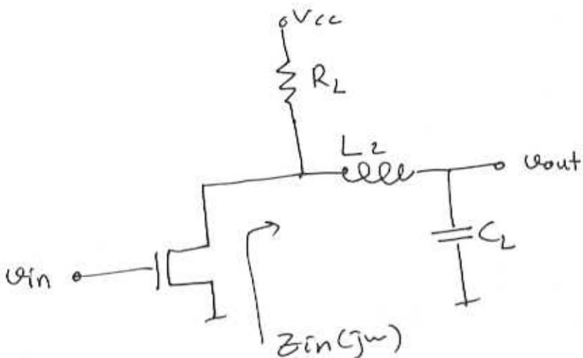
$$\text{Gain}(j\omega) = Z_{in}(j\omega) \cdot \frac{Z_C}{Z_C + Z_L} = G(j\omega)$$
