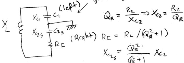
The circuit resonates at the frequency  $\omega_0$  defined by  $X_L + X_{C1} + X_{C2S}$
