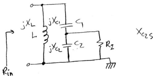
In this circuit we would like to find the impedance seen in parallel with the inductor, namely  $R_{in}$ . The problem is similar to  $\Pi$ -match, with the differences:
