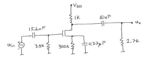
Estimate the lower 3dB cutoff frequency of the amplifier given above in cycles/sec. Note:  $g_{ni}$ = 10 millisiemens
