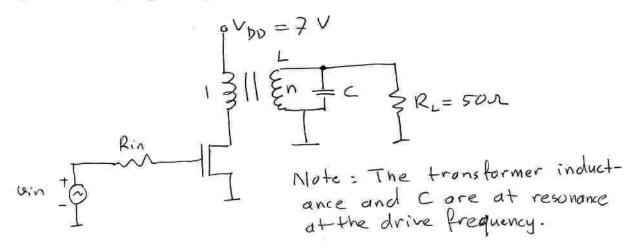
Given the Class A amplifier configuration above, we want to deliver 6 Watts into 50 Ohm load. The transistor is designed to operate with a supply voltage of 7 Volts.
