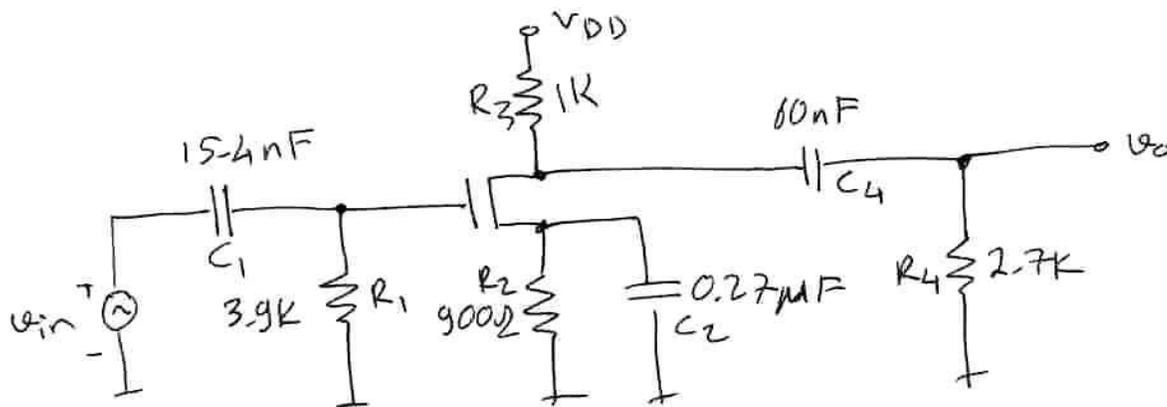
With the other capacitors short-circuited and of course  $v_{in}$  is short-circuited too, the resistance seen by  $C_1$  is  $R_1$ . Therefore:
