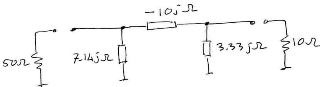
The actual component values, then can be determined if the operating frequency is given.
