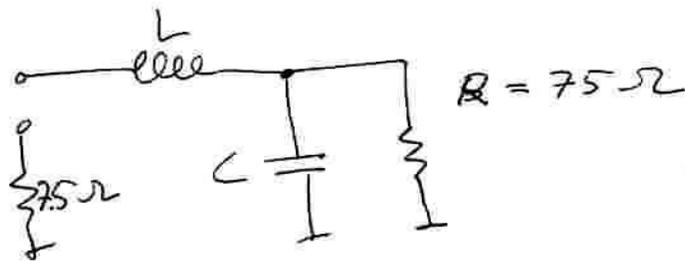
Since it should be lowpass the parallel component must be a capacitor to suppress high frequencies and the series component must be open circuit at high frequencies, too. Therefore it must be an inductor.
