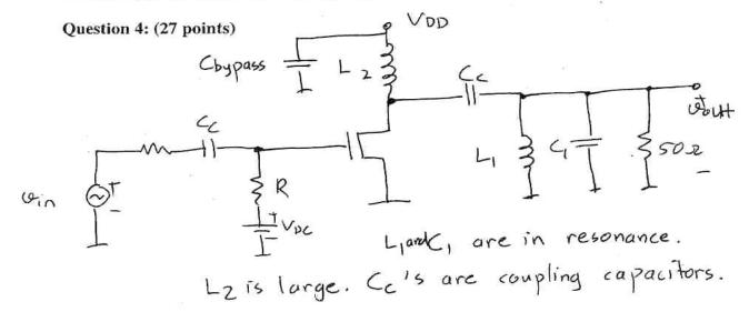
There is an RF power amplifier which was designed to operate either in class-A or class-B modes depending on the application. The delivered power is 1 Watts.
