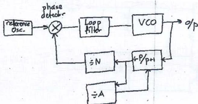
At the frequency synthesizer shown above  $f_{ref} = 2$  MHz. The N and A dividers are guaranteed to operate up to 500 MHz. The output frequency band of the synthesizer is 6-8 GHz. There are two prescalers available for design. They are divide by 6/7 and 16/17 prescalers. Choose the right prescaler and find a pair of N and A values to operate the frequency synthesizer at 6.5 GHz.
