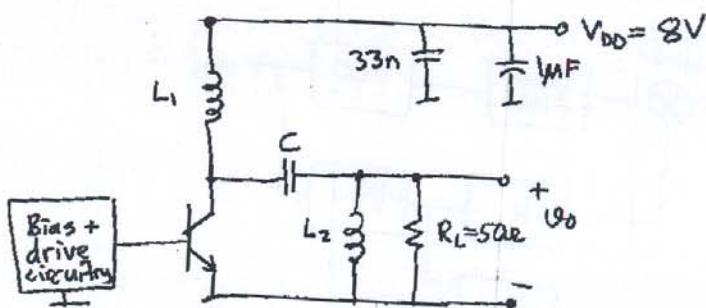
The circuit given above is operated as a class A amplifier at 100 MHz. In this circuit,  $V_{CESAT} = 1$  Volts and  $I_{max} = 1$  amps. Please carry out the following:
