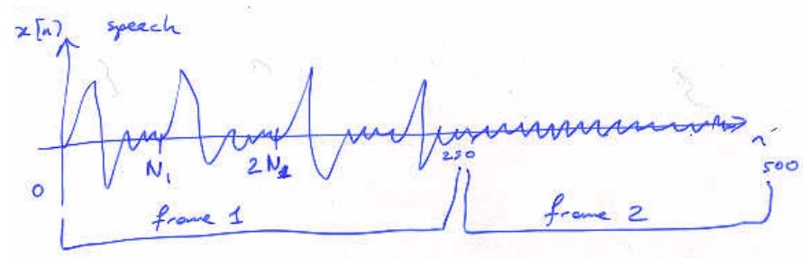
Fig. 8.14 Simplified speech model used in the LPC-10 algorithm
