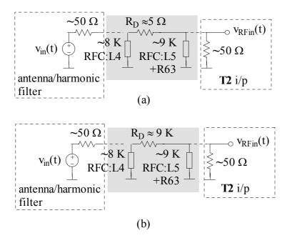
Figure 6.12 Equivalent circuit of RX RF attenuator at 16 MHz; (a) 10 mA bias current and (b) 14  $\mu$ A bias current
