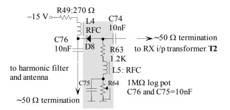
Figure 6.11 RX RF attenuator
