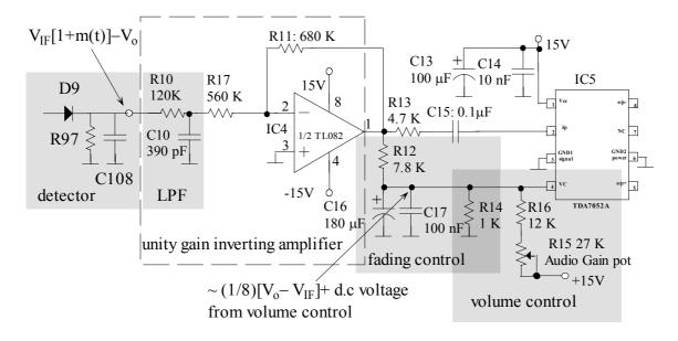
Figure 6.13 Audio gain control circuit
