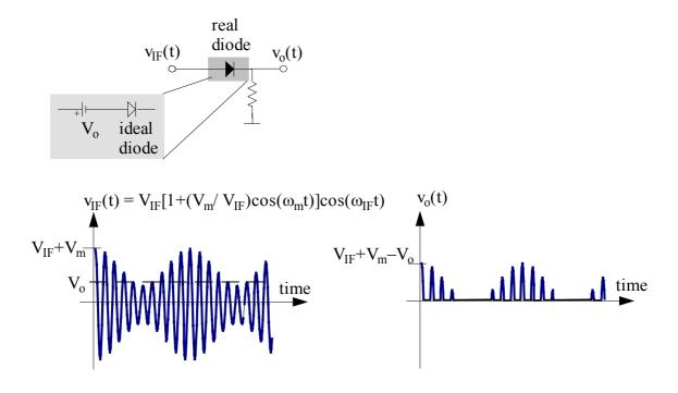
Figure 6.4 Rectifier with a real diode
