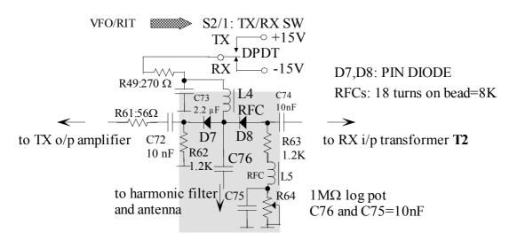
Figure 6.9 TX/RX switch circuit
