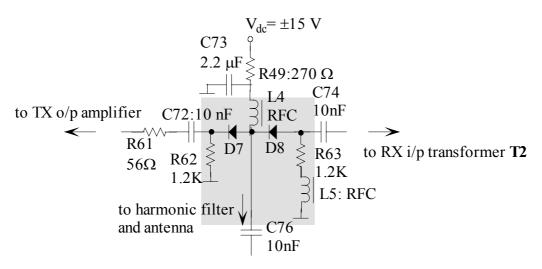
Figure 6.10 TX/RX RF switch circuit
