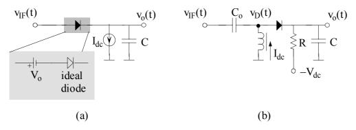
Figure 6.5 Envelope detector with a real diode compensated for  $V_o$ ; (a) equivalent circuit and (b) implementation
