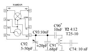
Figure 6.16 RX mixer input circuit
