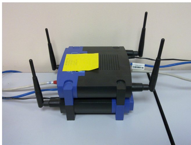
Fig. 2. A BilMesh two-radio node (Mesh Access Point) consisting of two distinct APs.
