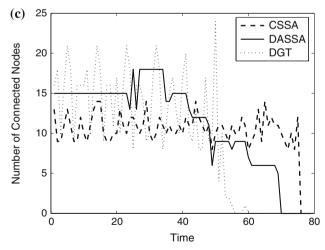
**Fig. 10** Energy and scheduling plots for GoC = 0.8 for the first topology; (a) Normalized total residual energy of all nodes with respect to 1 J. (b) Number of nodes which are dead at each round. (c) Number of nodes connected to the sink at each round
