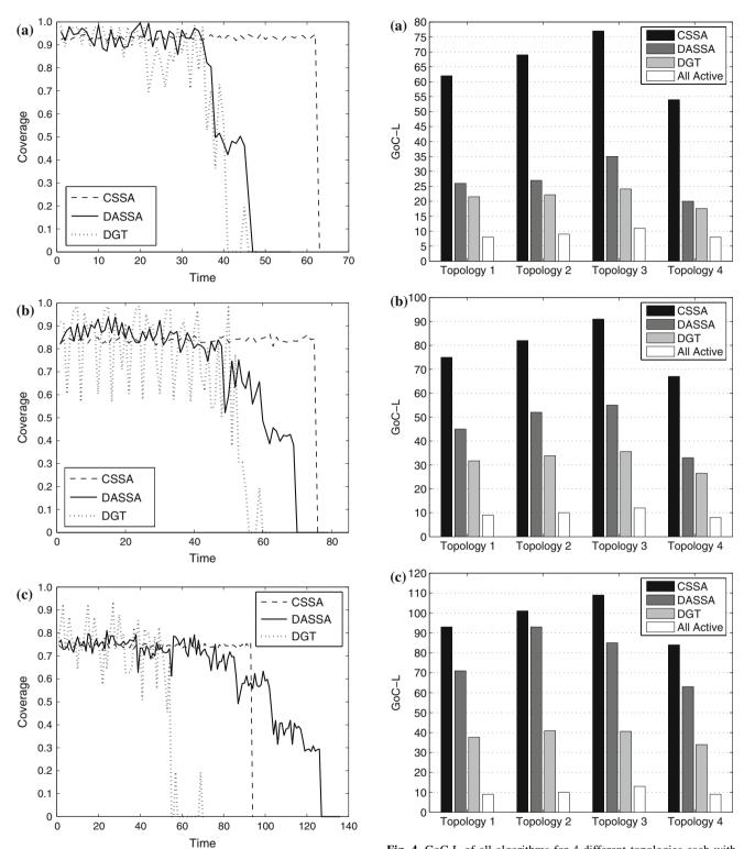
Fig. 3 CSSA, DASSA and DGT coverage plots for (a) GoC = 0.9, (b) GoC = 0.8, (c) GoC = 0.7
