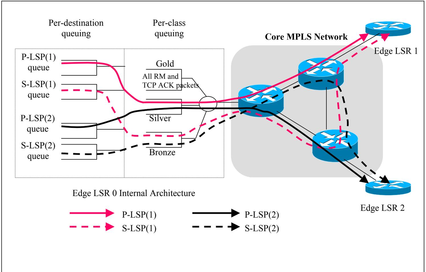
**Fig. 3** MPLS network with 3 edge LSRs and 3 core LSRs with strict priority queuing at the physical interfaces. All outgoing routes for edge LSR 0 for TCP data packets are depicted.
