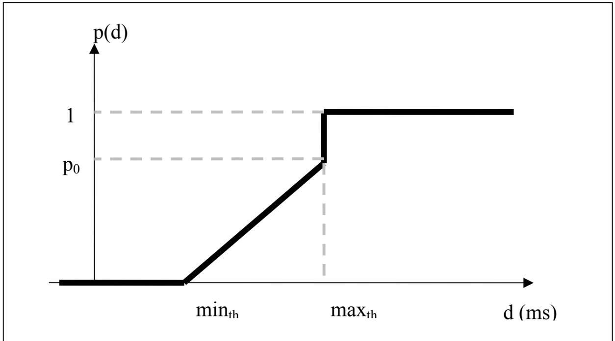
**Fig. 2** The traffic splitting function  $p(d)$
