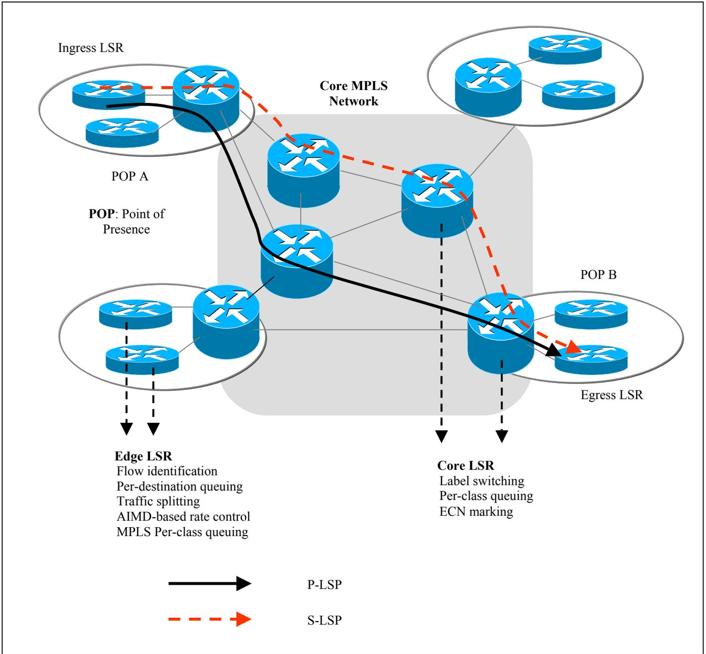
**Fig. 1** MPLS network with edge and core LSRs and the minimum hop P-LSP and the S-LSP from the ingress LSR at POP A to the egress LSR at POP B
