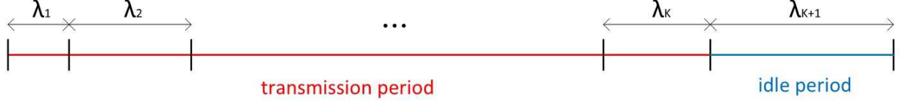
Fig. 2. A communication interval of T seconds during which channel switching is performed between the transmitter and the receiver. Communication occurs during the transmission period and stops during the idle period. \lambda_i shows the percentage of time channel i is employed for transmission with i \in \{1, \dots, K\} , and \lambda_{K+1} denotes the percentage of the idle period in the interval. The symbol rate of the communication link is assumed to be R in symbols per second.
