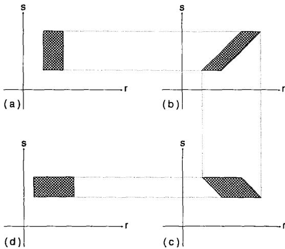
Fig. 7. (a) Phase space representation of the original bundle of rays. (b) After free space propagation through a distance  $f$ . (c) After passage through a lens of focal length  $f$ . (d) After another free space propagation through a distance  $f$ .
