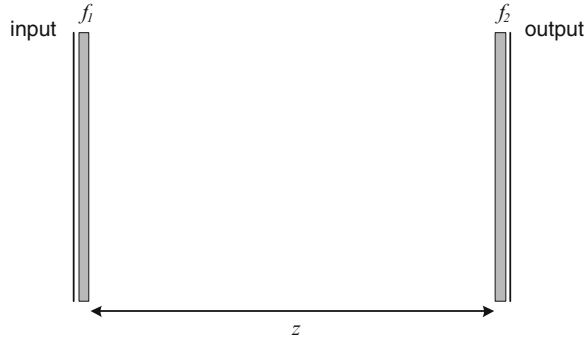
Fig. 6.2 Type-2 system which realizes arbitrary one-dimensional linear canonical transforms [36]
