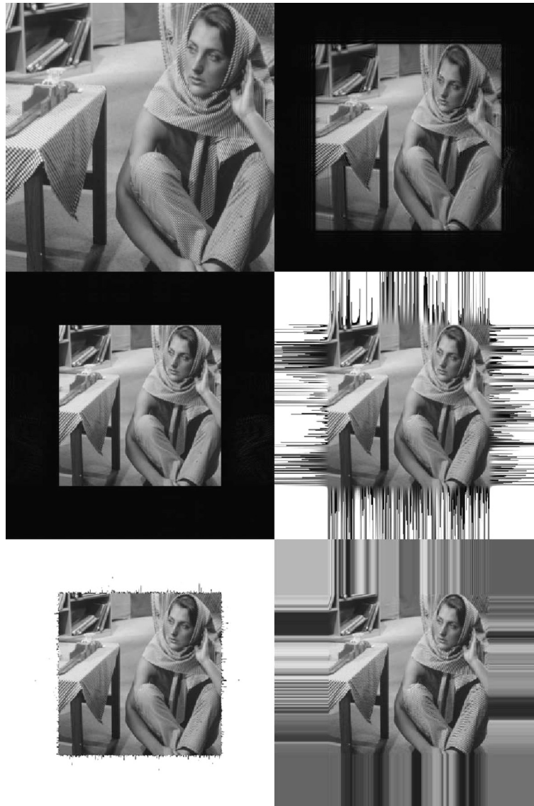
Fig. 3. Barbara. M = 0.6 . (From left to right; top to bottom: original, proposed (structural), proposed (formal), linear, spline, nearest).
