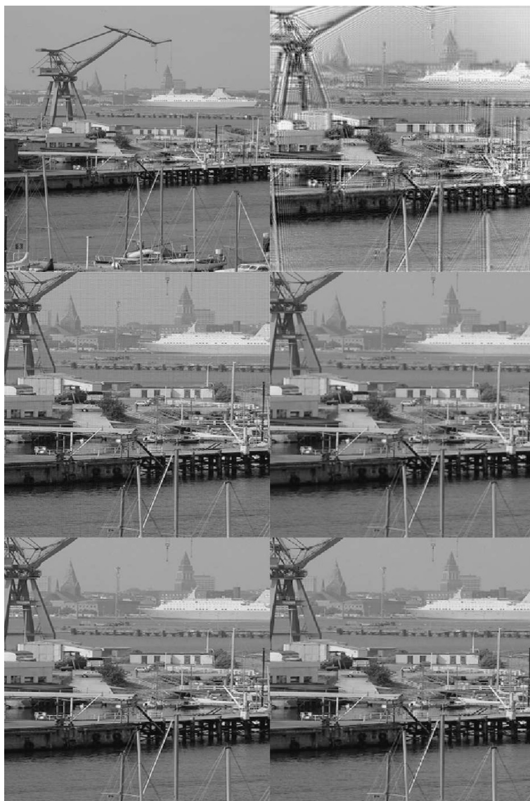
Fig. 7. Kiel Harbor. M = 1.6 . (From left to right; top to bottom: original, proposed (structural), proposed (formal), linear, spline, nearest).
