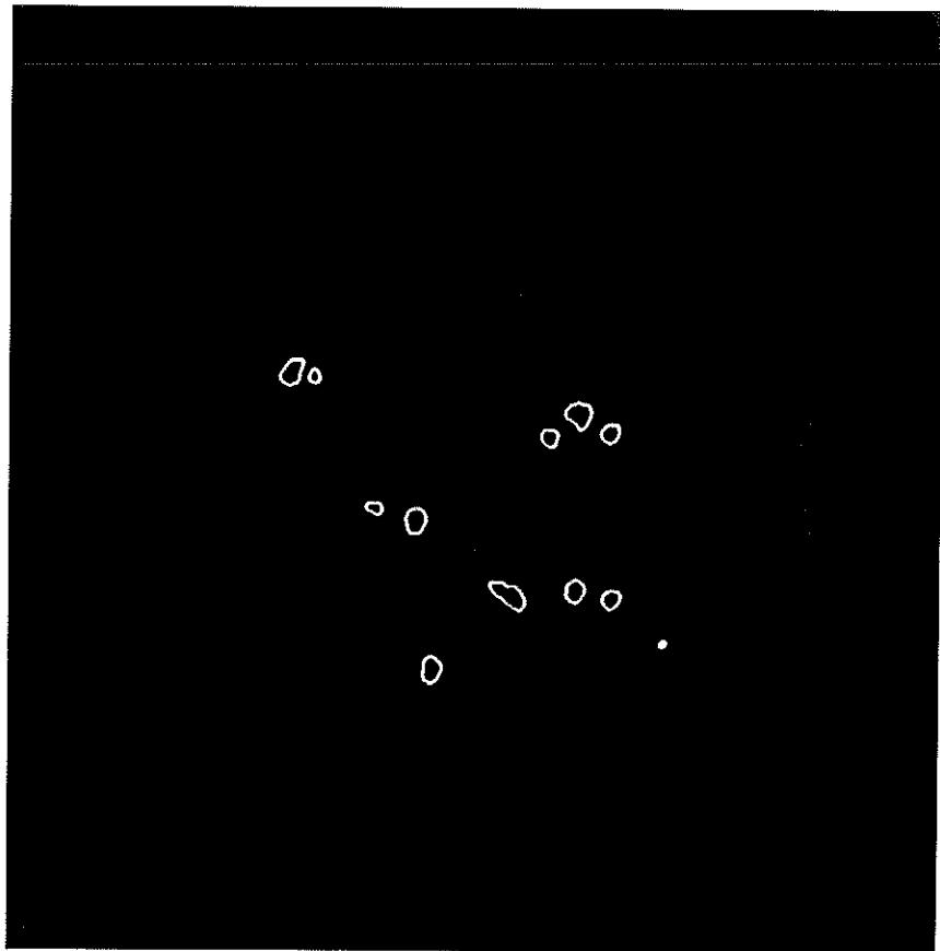
**Figure 51.** Result of covariance filtering applied to the reconstruction with twin-image elimination of Fig.43, after thresholding at gray level 128.
