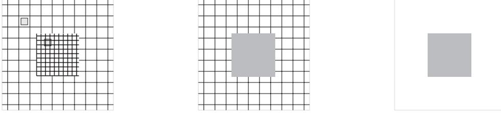
Figure 1: Example of the texture model showing a fine texture surrounded by a coarse texture (*left*). Result of application of opening (*middle*) followed by a closing (*right*).
