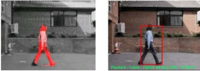
Figure 1. Moving pixels (left) and their minimum bounding boxes are determined.
