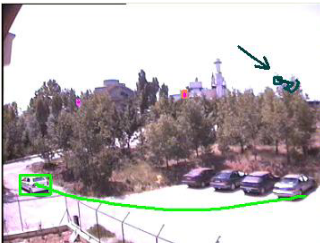
Figure 2. The car has a directionally consistent trajectory whereas the leaves, pointed with an arrow, sway randomly in the wind.
