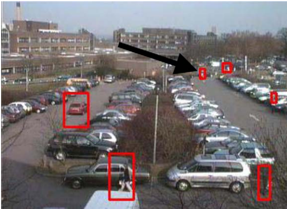
Fig. 6. Detection result of the subband domain method using all of the 3 rd level wavelet coefficients. Walking man marked as MAN1 is pointed.
