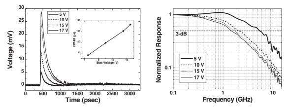
**Fig. 3** a) Bias-dependent temporal pulse responses of an AlGaN MSM PD with 3  $\mu$ m finger spacing. Inset shows the measured FWHM values with respect to bias voltage. b) Corresponding FFT curves with 3-dB bandwidths of 5.4, 2.1, 1.7, and 1.5 GHz at 5, 10, 15, and 17 V bias respectively.
