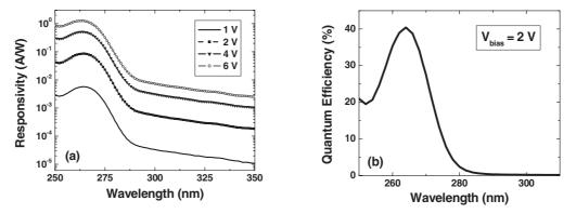
**Fig. 2** a) Measured spectral responsivity curves of AlGaN MSM PDs as a function of bias voltage. b) Linear-scaled plot of the corresponding spectral quantum efficiency under 2 V bias.
