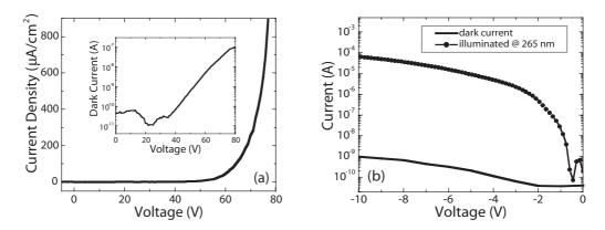
Fig. 1 a) Dark current density of an MSM-PD with 10  $\mu$ m finger spacing. Inset shows the leakage current in logarithmic scale. b) I–V curves of a device with 5  $\mu$ m finger spacing under different illumination conditions.
