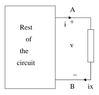
• Reference Directions : Two nodes are required for voltage, and a terminal is needed for a current. If, after calculations voltage/current turns out to be **positive**  $\rightarrow$  the chosen reference directions are right, otherwise wrong.
