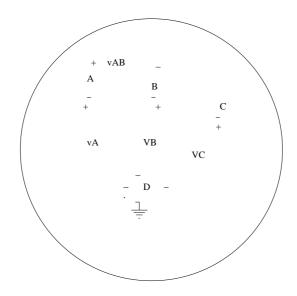
The voltage between any node and ground node is called node voltage
