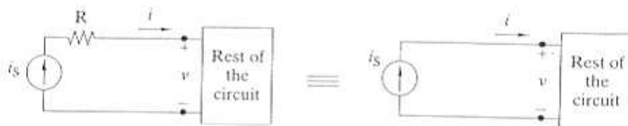
FIGURE 2-33 Equivalent circuit of a current source and a resistor in series.
