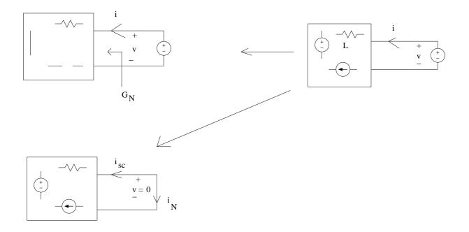
• Because of unique solvability, we can replace N by a voltage source (this is called substitution). This circuit is uniquely solvable. Hence apply superposition :
