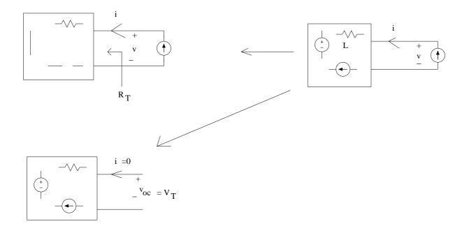
• Because of unique solvability, we can replace N by a current source (this is called substitution). This circuit is uniquely solvable. Hence apply superposition :
