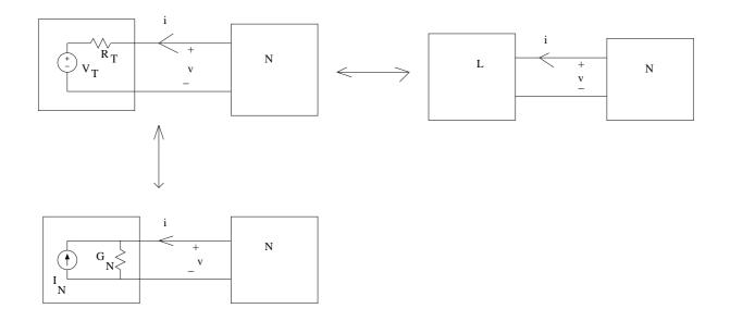
•  $v_T$ : Thévenin equivalent voltage source,  $R_T$ : Thévenin equivalent resistance,  $i_N$ : Norton equivalent current source,  $G_N$ : Norton equivalent conductance.
