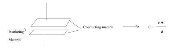
$\bullet$  Here A is the area, d is the distance between plates, and  $\epsilon$  is the dielectric constant of the insulating material.
