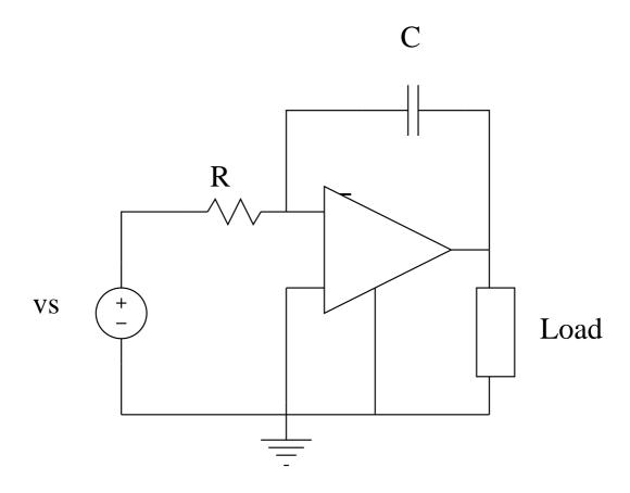
$$\bullet \ v_- = v_+ = 0 \rightarrow v_s = Ri_R \ , \ v_C = -v_0$$
