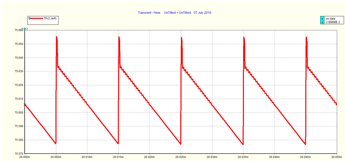
Plot : v_{out}(t) vs. t for 20ms to 20.05ms duration. We waited till 20ms to reach steady state. v_{out,max} = 75.655 \text{ V} and Ripple Voltage (Peak-to-peak) equals to 75.654 - 75.578 = 76 \text{ mV} .
