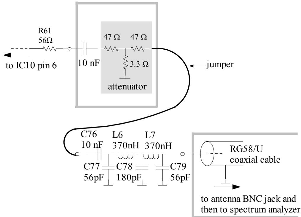
Figure 5.22 Harmonic measurement set up
