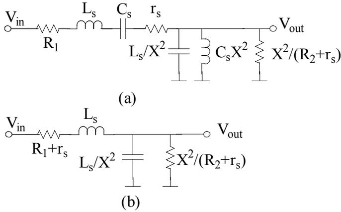
Figure 5.19 (a) Equivalent circuit of two-crystal ladder BPF and (b) LP equivalent of the filter
