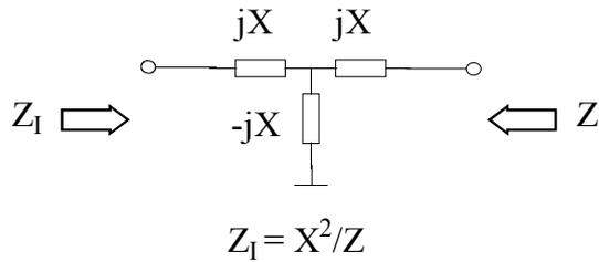
Figure 5.16 Impedance inverter
