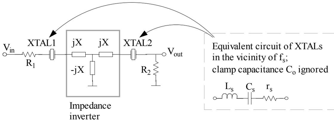
Figure 5.18 Two-crystal ladder filter
