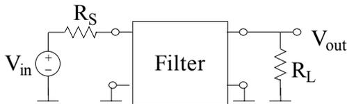
Figure 5.1 Electronic filter
