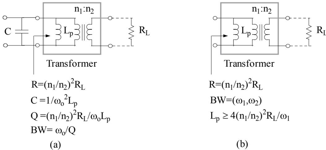
Figure 5.13 (a) Narrow-band transformer, (b) Wide-band transformer
