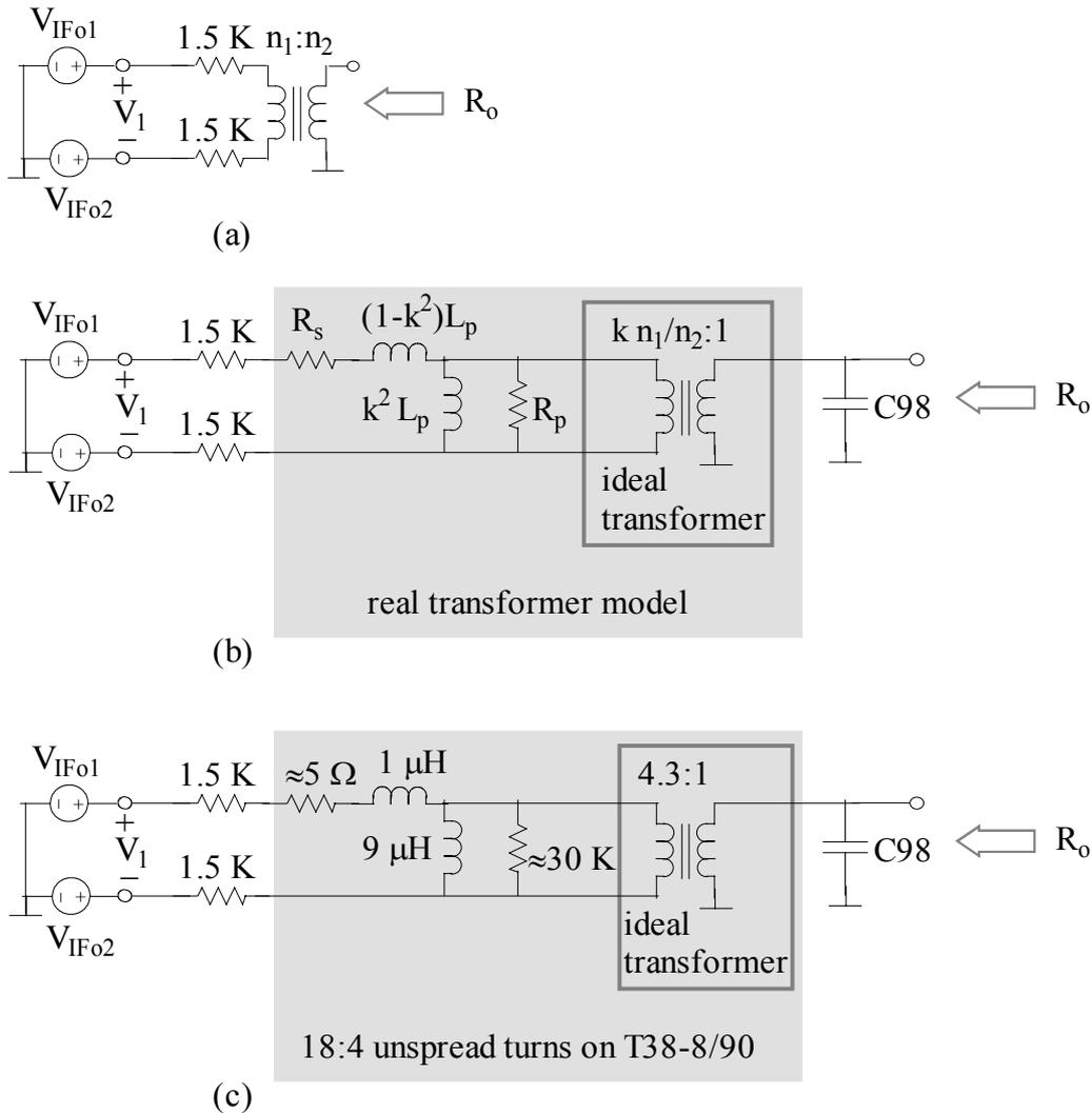
Figure 5.25 Impedance matching between RX mixer and IF filter (a) with an ideal transformer, (b) with a real tuned transformer model and (c) with the typical values of a transformer with 18:4 turns on a T38-8/90 toroid core.
