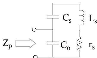
Figure 5.31 Quartz crystal equivalent circuit
