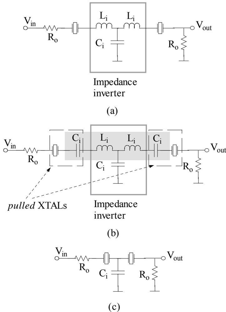
Figure 5.20 Impedance inverter for two-crystal ladder filter, (a) Proper inverter, (b) Inverter inductors tuned out by series capacitors, modifying the series XTAL branches, (c) Actual circuit with only one capacitor
