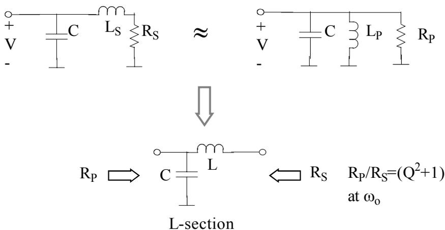
Figure 5.15 Narrow band impedance matching using L-section filters
