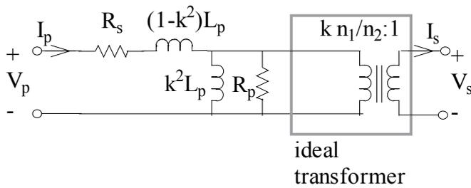
Figure 5.14 Equivalent circuit of a real transformer.
