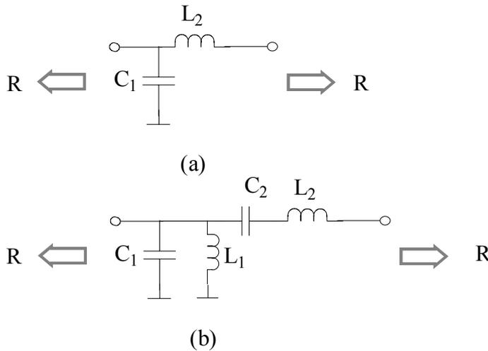
Figure 5.9 (a) LPF with  $\omega_c = \Delta\omega$ , (b) BPF obtained by tuning out  $C_1$  with  $L_1 = 1/\omega_0 C_1$  and  $L_2$  with  $C_2 = 1/\omega_0 L_2$
