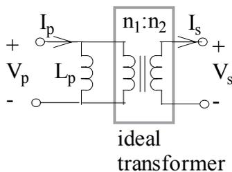
Figure 5.12 Equivalent circuit of a lossless real transformer
