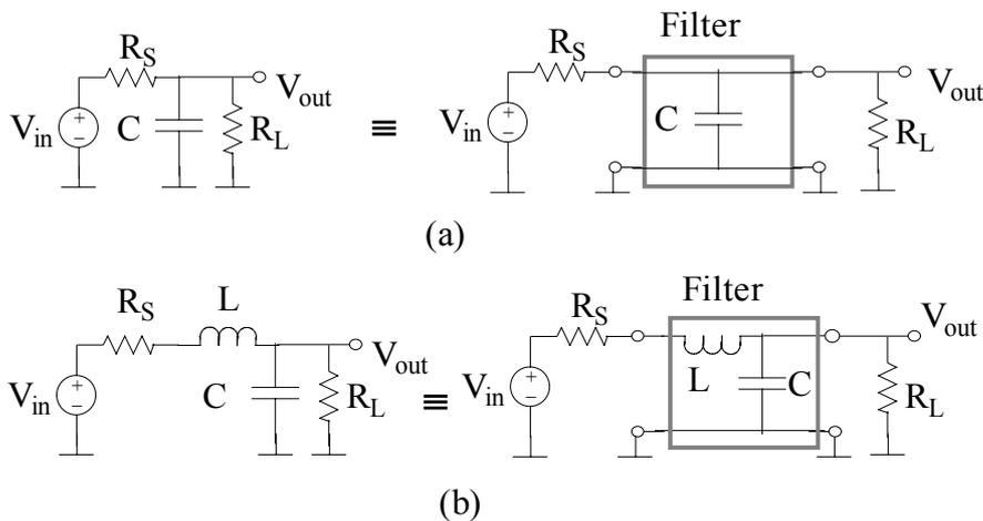
Figure 5.2 LPF (a ) one element, (b) two elements
