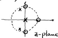
(c) The zeros of the numerator polynomial are on the unit circle at  $Z=e^{j0}$ ,  $Z=e^{j\pi/2}$  and  $Z=e^{j\pi/2}$  when  $x[n]=Ae^{j\phi}e^{j\hat{\omega}n}$ , the output y[n] is  $y[n]=H(e^{j\hat{\omega}})\cdot Ae^{j\phi}e^{j\hat{\omega}n}$  There the output will be zero when  $H(e^{j\hat{\omega}})=0$ . That is, for  $\hat{\omega}=0$ ,  $\hat{\omega}=\pi/2$  and  $\hat{\omega}=-\pi/2$ .
