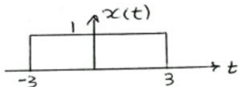
$$T_{0/2} = 3 \rightarrow X(j\omega) = \frac{\sin(3\omega)}{\omega/2}$$
