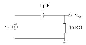
Measure the output voltage for 1 KHz, 10 KHz, 100 KHz, 1 MHz sine-wave input waveforms ( $v_{pp} = 1 V$ ). Connect the X probe of the scope to  $v_{in}$  and Y probe of the scope to  $v_{out}$  and observe both waveforms on the screen. Repeat this for the X - Y mode.
