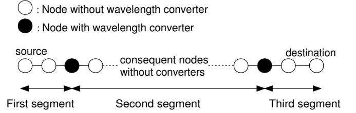
Fig. 1. Division of a lightpath into segments
