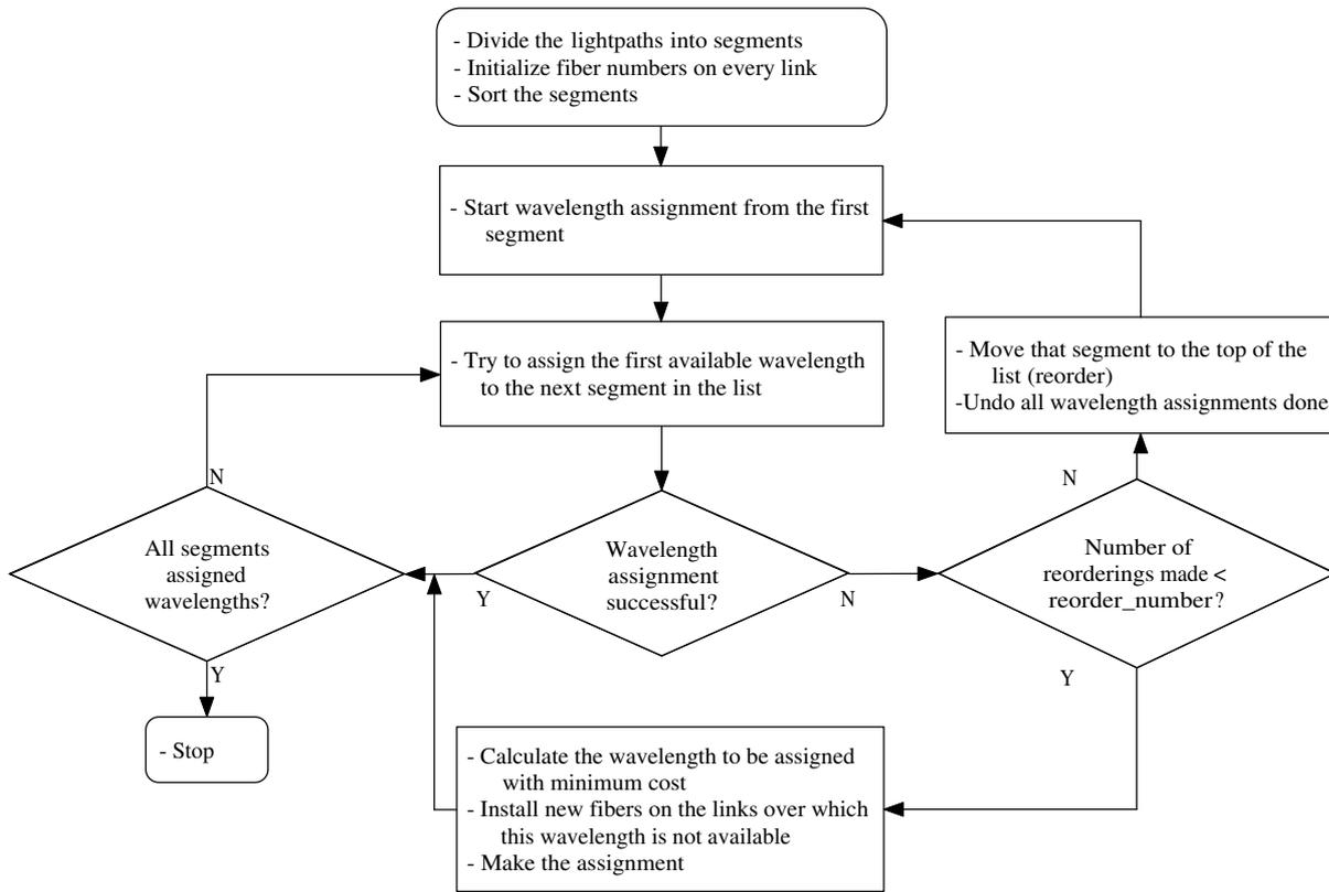
Fig. 2. Flowchart of the RLPF wavelength assignment algorithm
