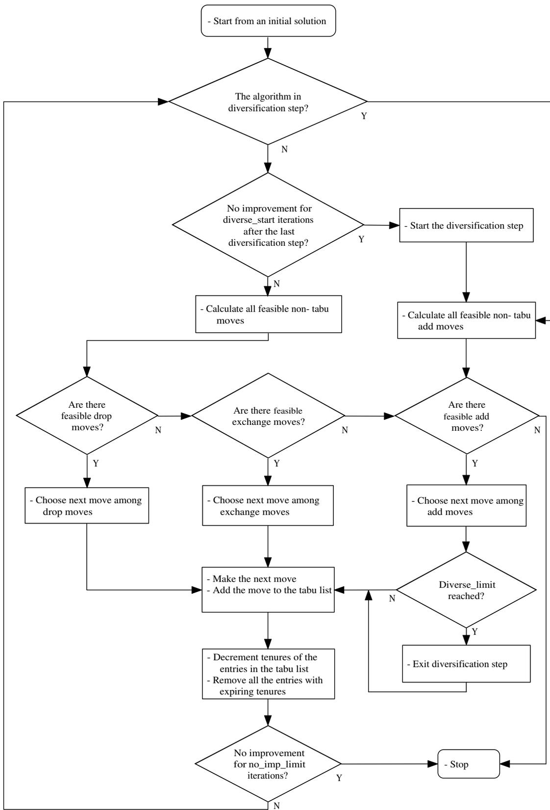
Fig. 3. Flowchart of the TSCP algorithm
