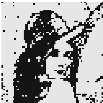
Figure 3: Classification of image blocks of “Lenna” into groups of high and low activity. Grey pixels represent low-activity blocks and black pixels represent high-activity blocks.
