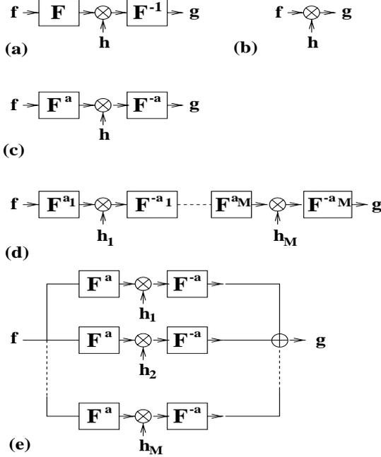
Figure 1: Single-stage filtering in the Fourier domain (a), the time domain (b), and the  $a$ th order fractional Fourier domain (c). Multi-stage (repeated) filtering (d). Multi-channel (parallel) filtering (e).
