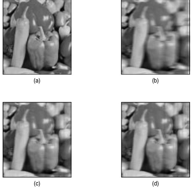
Figure 3: Original image (a). Blurred image (b). Restored by repeated filtering ( $M = 5$ ) (c). Restored by multi-channel filtering ( $M = 5$ ) (d).
