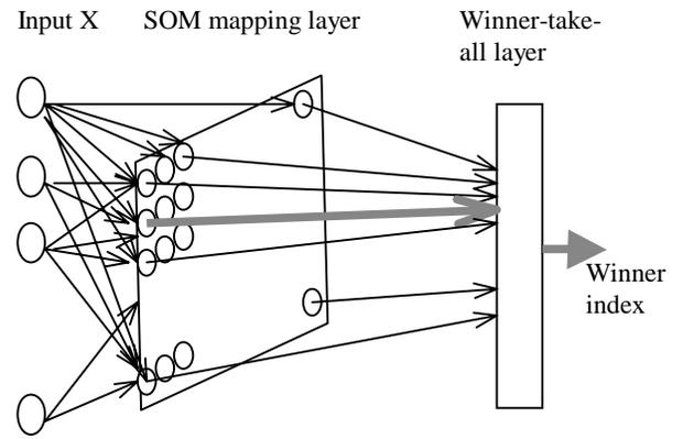
Fig. 5 Self-Organizing Map neural network with time frequency vector as input
