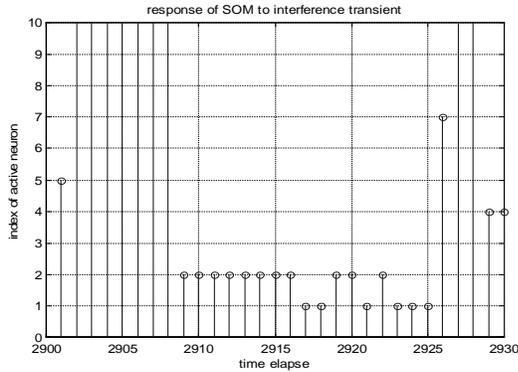
Fig. 8 Index of active neuron corresponding to interference transients
