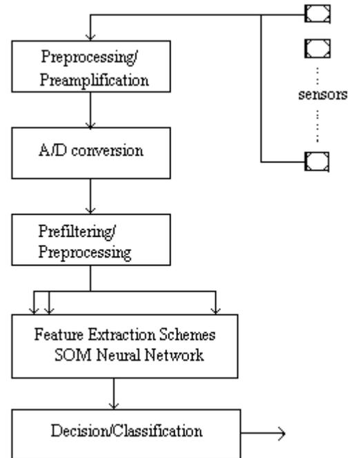
Fig. 2 Transient Classification System Block Diagram
