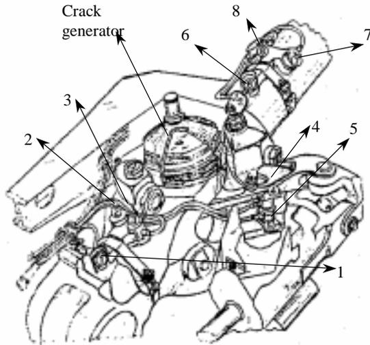
Fig. 1 Sensor position at in-flight data acquisition system
