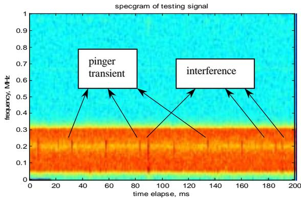
Fig. 4 Spectrogram of a segment of data from sensor 2
