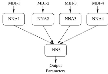
Figure 2: Fusion of MBI using Multilayer Neural networks
