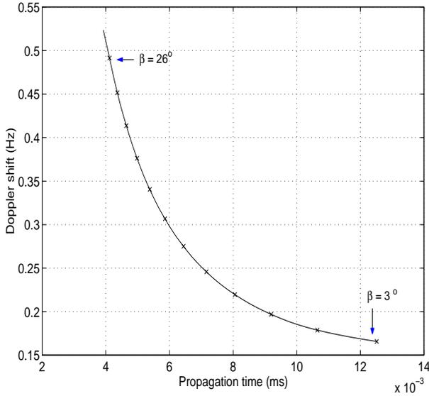
Figure 1: Example of Delay-Doppler function for 12 elevation angles
