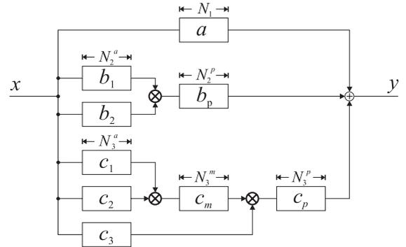
**Figure 1.** Approximation of a 3<sup>rd</sup> order Volterra series expansion with a MMD-filter structure
