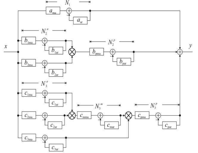
**Figure 2.** MMD-ARMA filter structure based on linear ARMA filters and multipliers
