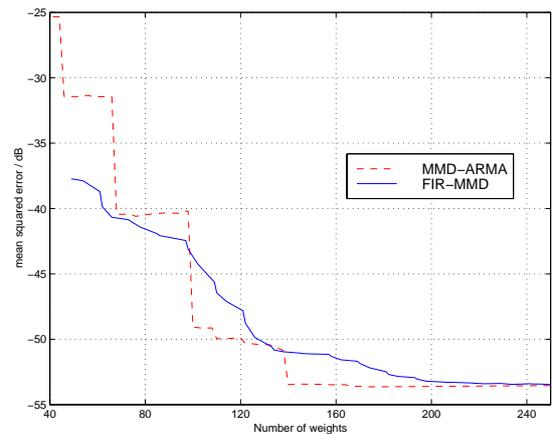
Figure 4. Comparison of effort between FIR-MMD and MMD-ARMA. Basically the MMD-ARMA structure needs a lesser number of filter weights.
