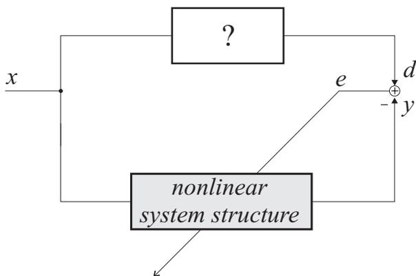
Figure 3. Structure for identifying nonlinear systems
