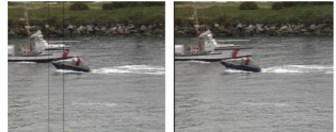
Figure 5. Performance of the LSSI interpolator: Left- Line Scratch degraded image; Right- Restored image
