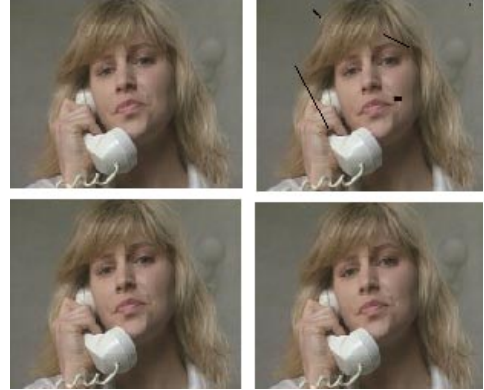
Figure 4. Performance of the ML3Dex interpolator: Top Left- Original non-degraded image; Top Right- Blotch degraded image; Bottom left- Restored image using the correct mask of defects. Bottom right- Restored image using the mask of defects produced by the SDI_S .
