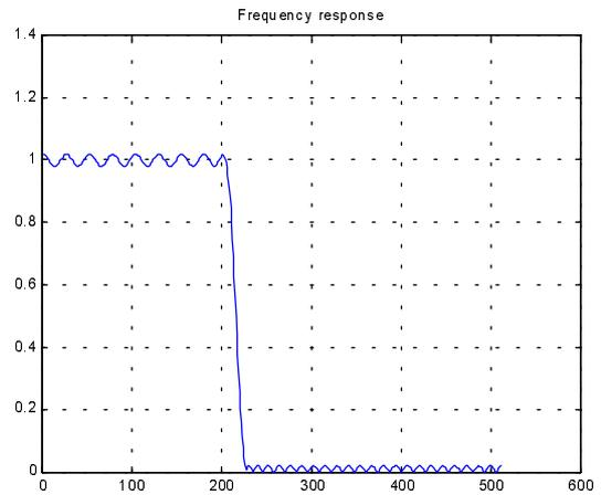
Figure 2: Amplitude response of the original linear phase FIR filter transfer function.
