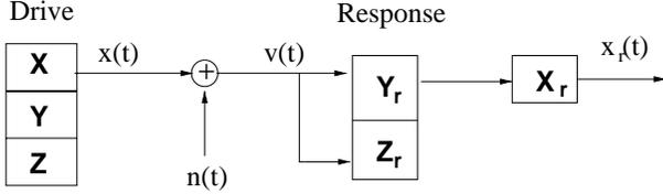
Figure 1: Drive-response synchronization schematic diagram.
