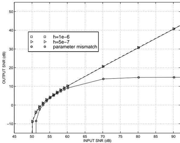
Figure 3: Synchronization performance using Ito / Mannella and Palleschi method( $K = 2505$ ).
