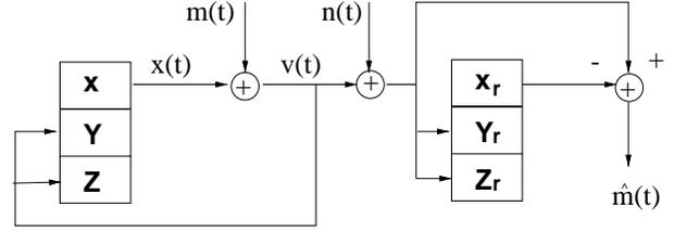
Figure 6: Dynamic feedback modulation communication system.
