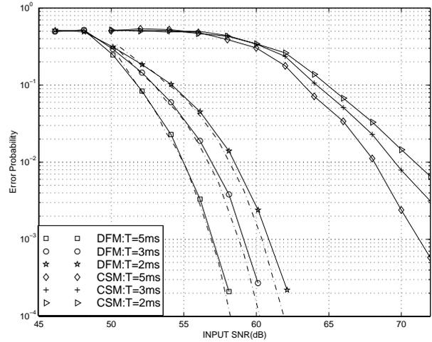
Figure 7: Chaotic communication system performance for DFM and CSM ( $K = 2505$ ).
