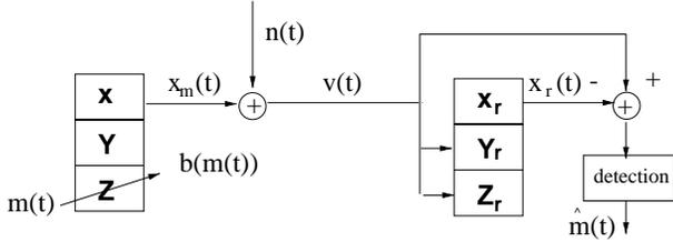
Figure 5: Chaotic switching modulation communication system.
