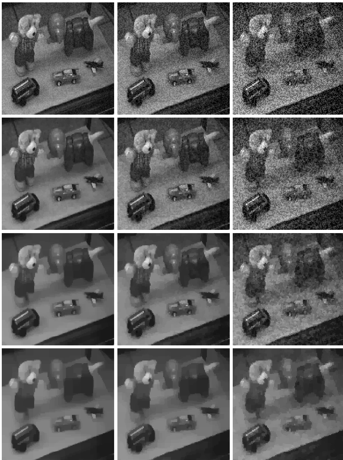
Figure 4. Comparison of three restoration of images with three noise levels (original image is shown in the bottom left of Figure 3.) Each column shows input (top row) and restoration using three smoothing constant \mu 's; \mu=6 (second row), \mu=20 (third row), and \mu=40 (bottom), where F(x)=\mu|x| .
